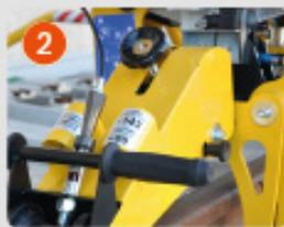
Machine settings are achieved without tools and rear arms have protection against damage with adjustable gas springs for assured machine lifting in all weather.
