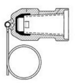
**Wedge for CB/CC.** Dismantling wedge is used to ventilate into the air when removing the rear plug in shielded connectors. 1 pcs. El no. 88 402 33
