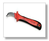
**HB9.** Insulated knife with curved blade and protective cover. Suitable for insulation and screen removal, equipped with blade guide to avoid damage to strands.
