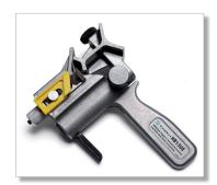
**HB13UE.** Universal cable stripping / splitting tool for outer jacket on low and medium voltage cables Ø 12.7 to 63.5 and XLPE primary insulation max. Ø 38.1mm.
